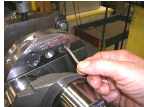
Insertion of Circlip Check Gage
