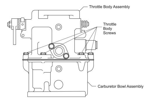
Models MA-3A, MA-3PA, MA-3SPA, and MA-4SPA have four screws. Models MA-4-5, MA-4-5AA, and MA-6AA have six screws.
