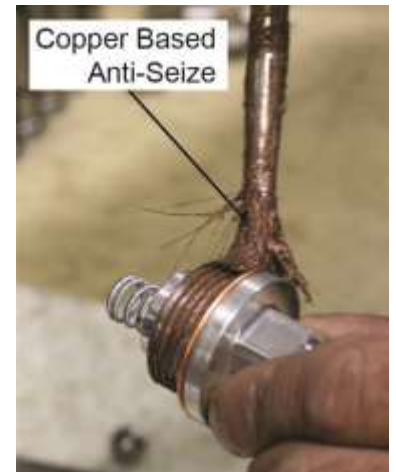
Figure 6 Apply Copper Based Anti-Seize to Threads
