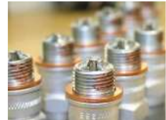
Figure 4 Copper-Based Anti-Seize Applied to Spark Plug Threads
