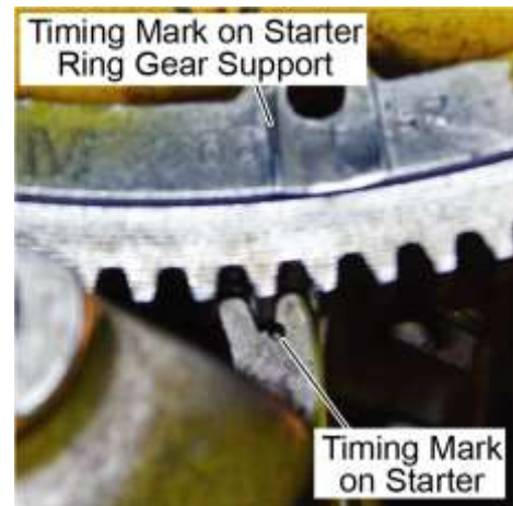
Figure 9 Timing Marks on the Propeller Side of the Starter Ring Gear Support Aligned with the Timing Mark on the Starter
