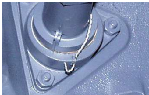
Figure 2 Safety Wire on the Oil Level Gage
