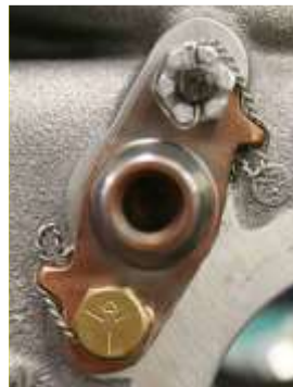
Figure 17 Safety Wire on the Idler Gear Shaft
