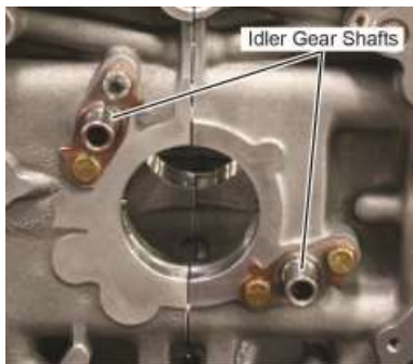
Figure 59 Shaft Installation in the Crankcase for Left and Right Crankshaft Idler Gears
