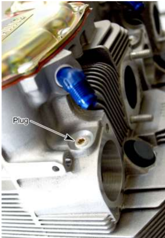
Figure A-8 Plug Above the Intake Port
