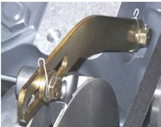
Figure 4 Safety Wire on Bolts of Alternator Adjusting Link
