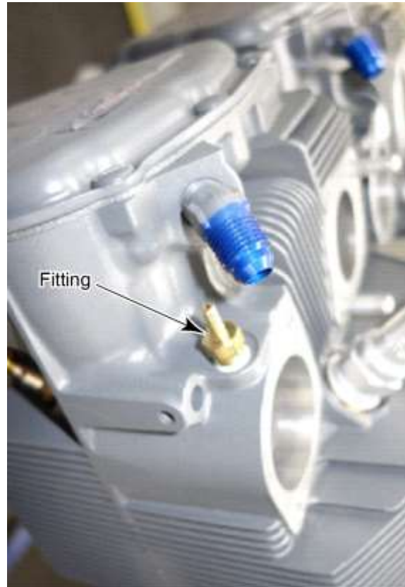
Figure A-9 Fitting Installed in the Cylinder
