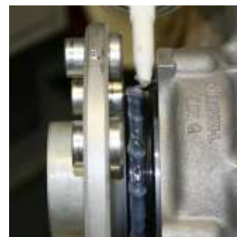
Figure 92 Apply the Sealant to the Oil Seal
