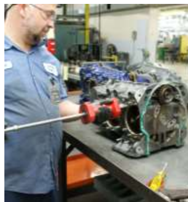
Figure 5 Strike the Slide Part of the Tool Against the Back of the Tool
