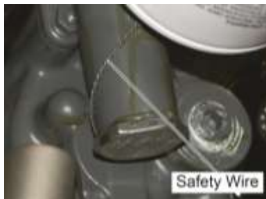
Figure 7 Safety Wire on the Oil Cooler Bypass Valve:
