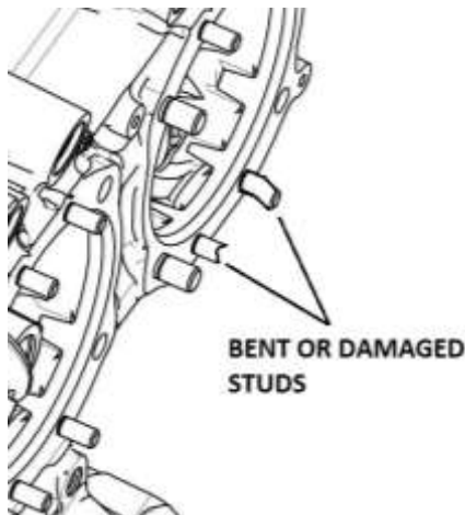
Figure A-1 Damaged Studs
