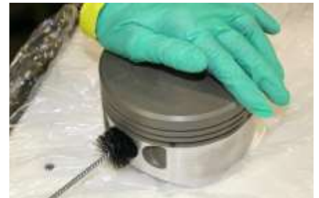
Figure 2 Cleaning the Piston Pin Bore with a Soft Bristle Non-Metallic Brush
