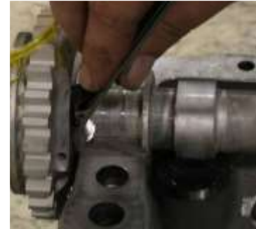
Figure 74 Camshaft End Play Clearance Check
