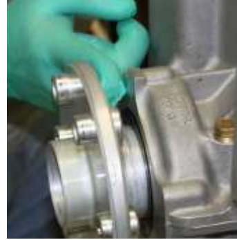
Figure 93 Spread the Excess Sealant
