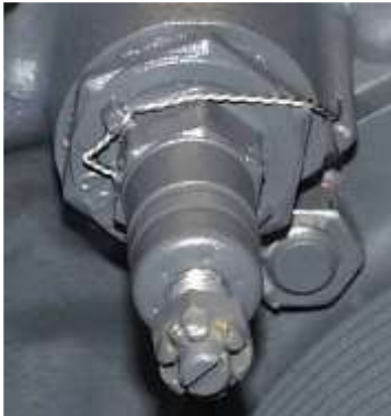
Figure 4 Safety Wire on the Oil Pressure Relief Valve
