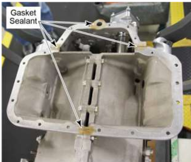
Figure 15 Gasket Sealant# 4 (or Equivalent) to Three Places on Oil Sump
