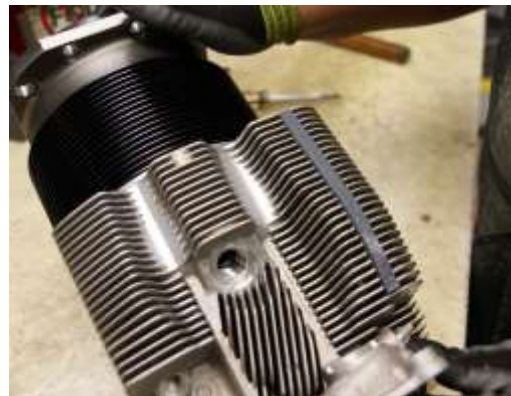
Figure A-5 Fin Stabilizer Installed on Cylinder
